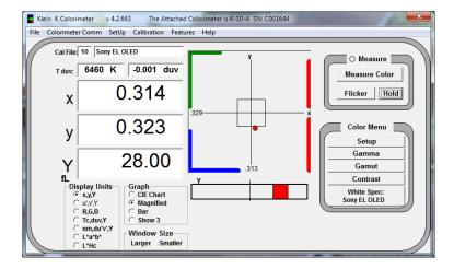
**Correction Method #1:** As a solution we can change the target white spec stored in the K10's Sony OLED cal file. Instead of the REC709 target white xy values of (0.3127, 0.3290), offsets are subtracted and the white point target becomes (0.3117, 0.3240). This is modified in the K10 white spec for this particular display in the K10 flash.
