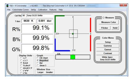
You have completed the procedure for modifying the white point spec in the Sony OLED cal file. That white target spec is now stored in the K10 flash and will be loaded to the K Colorimeter program each time the Sony OLED cal file is recalled.
