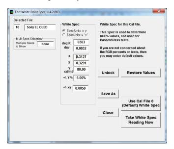
Press the "Unlock" Button and enter the new xy values for the Sony White Point (0.3117, 0.3240):
