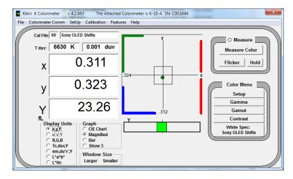
And.. as always, if adjustments on your display are to be made in RGB units, then the easiest (non-interactive between colors) method of adjustment is using the RGB% Display Units. When the three % match one another, then xy is proper, and when the three values are at 100%, the display is also adjusted to the white spec Y value.
