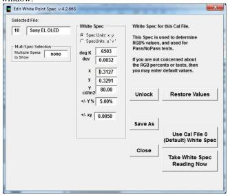
Instead of entering the modified values by keyboard, use the "Take White Spec Reading Now" button to record the current xy values as the new white point spec. The other steps are the same as above.
