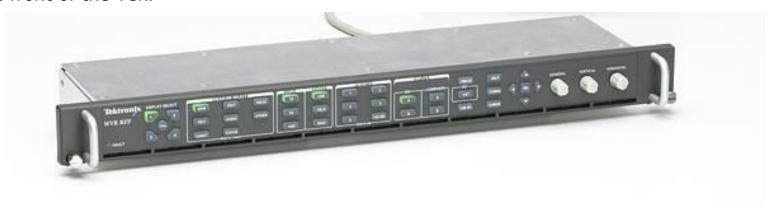
The five present buttons on the front act to recall a preset when pressed momentarily, but if you hold in the button for three seconds that preset records the entire state of the machine. So, get the instrument exactly as you want it – what displays are in the four tiles, what parameters are being monitored etc and then store it away. You can download and upload preset templates over the web interface or via a USB stick on the WFM-version.
