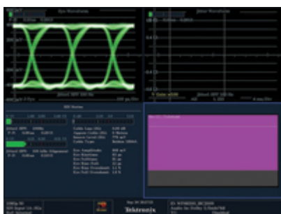
Figure 2. Testing video coax cable at 3Gb/s Select figure to enlarge.
