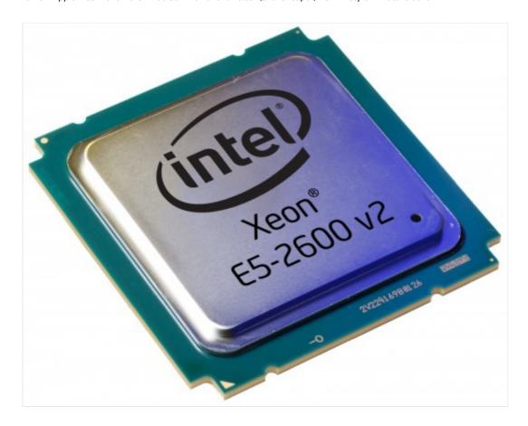
Intel's Xeon E5-2697 V2 is an Ivy Bridge-E part with over 12 cores, riding within a 130 watt TDP. With 30MBs of L3 cache, this is definitely, spec for spec, the chip that is in the top end Mac Pro. Whether it's chip is soldered to the board, or at least, has the cap pulled off like in the previous Mac Pros, is still unknown. As mentioned, this may or may not be an unknown quantity in our chosen motherboard as it might not be fully compatible.
