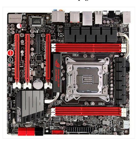
In order to get support for the higher core count processors, an LGA2011 socket board was needed. But even more than that, in order to fit it in inside the Silverstone FTo3 (or SG10) you'd need a micro ATX board. The only board that seems to fit the bill is the ASUS Rampage IV Gene from their ROG line up. It also seems to be the only board left on the market that hasn't been discontinued and ASUS does offer extremely good support for their flagship ROG parts even at end of life.
