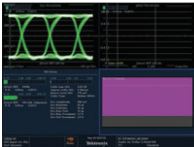
Figure 2. Testing video coax cable at 3Gb/s Select figure to enlarge.
